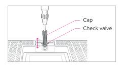
Figure 5. Actuating the check valve in the top accumulator on the 192.24 IFC
