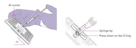
Figure 6. Injecting control line fluid into the accumulators on the 192.24 IFC
